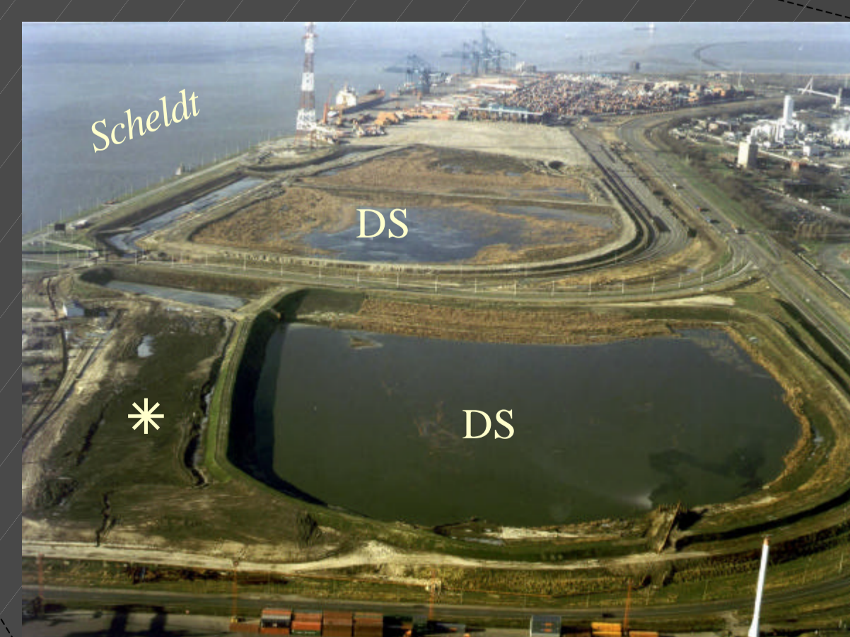
▶ Figure 2. Aerial view of the disposal sites (DS) near Magers-hoek. The experimental dike (*) was constructed with consolidated dredged material from the disposal site in front of the picture. The locks of Berendrecht and Zandvliet are at the left of this picture (not visible). (Foto: verzameling Gemeentelijk Havenbedrijf - HB/TD).
